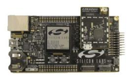
Mainboard (BRD4001) which feature an on-board J-Link debugger, an Advanced Energy Monitor for real-time current and voltage monitoring, a Virtual COM port interface, and access to the Packet Trace Interface (PTI).
